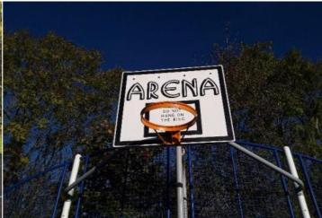
Finding: A clearly visible facility sign should be provided in Action: Provide signage to BS EN 15312 a prominent position with the wording as detailed BS EN 15312- the equipment is not intended for children less than 3 years old- the warning - Do not climb on the framework or nets- the warning - Do not hang on the ring (if provided)- the warning - Do not wear rings or other jewellery- name and telephone number of the administrator- number to call in case of accident
