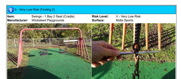
**Finding:** The chain openings are in excess of the 8.6mm as **Action:** Monitor - No remedial work recommended recommended by BS EN 1176
