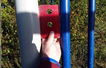
**Finding:** The item fails to meet the requirements of BS EN 15312 4.4.2.1 head and neck entrapment in the framework
