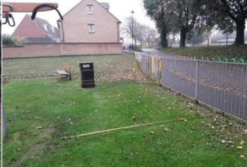
Finding: BS EN 1176 Part 5 states that for Type C Carousels, an additional obstacle free space of at least 1.0m shall be provided from the edge of the free space / impact area and there is insufficient obstacle free space provided
