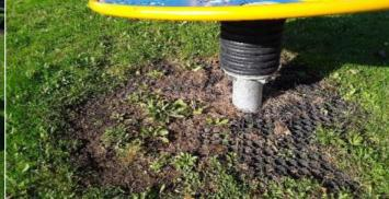
Finding: The bearing is showing signs of wear
