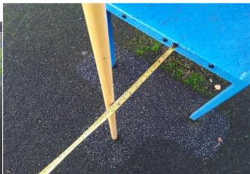
**Finding:** The free space between the fireman's pole and the **Action:** Monitor - No remedial work recommended platform is less than the minimum recommended dimension of 350mm in BS EN 1176 Part 1; this is however an intended design feature by the manufacturer to assist younger users in accessing the pole and is a very low risk finding - no remedial action is recommended
