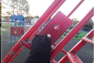
Finding: The item fails to meet the requirements of BS EN Action: Monitor - No remedial work recommended 1176 Part 1 4.2.7.2 head and neck entrapment in the
